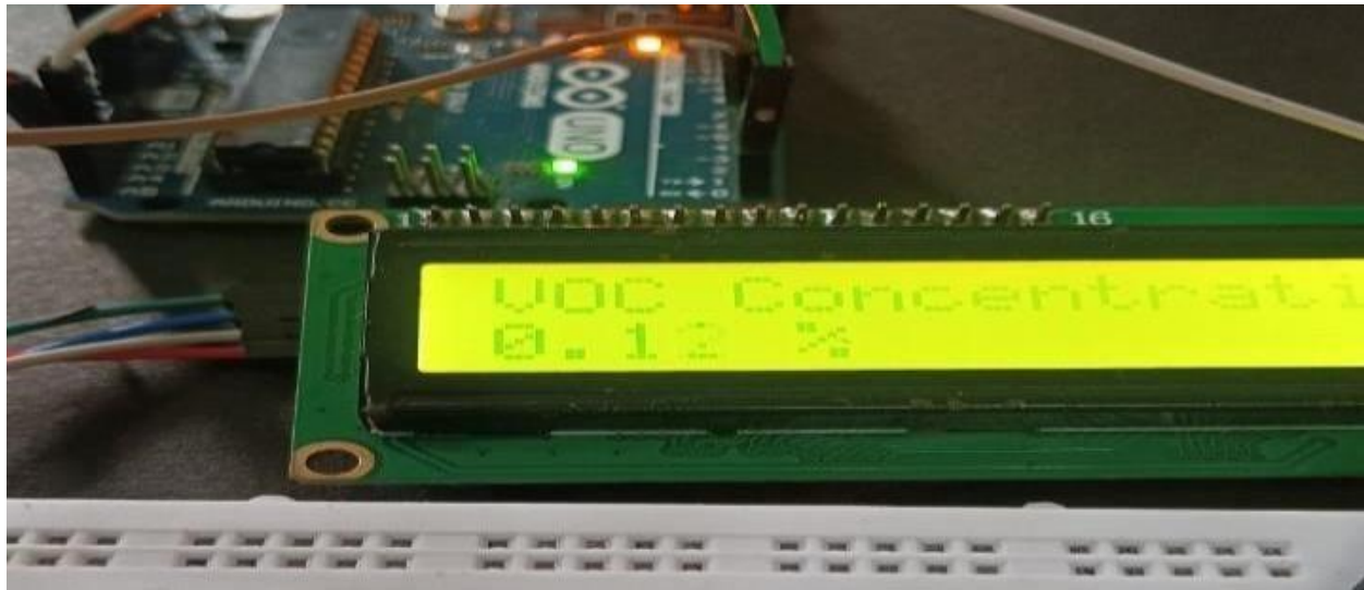
Figure 15: 7.4 LCD Display when ethanol is detected
