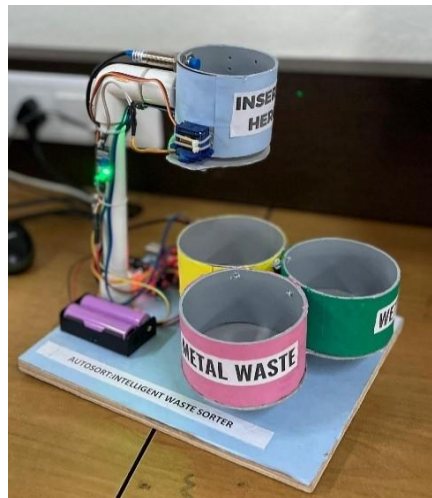
Figure 7: 7: Working prototype of Auto-sort Intelligent Waste Sorter
