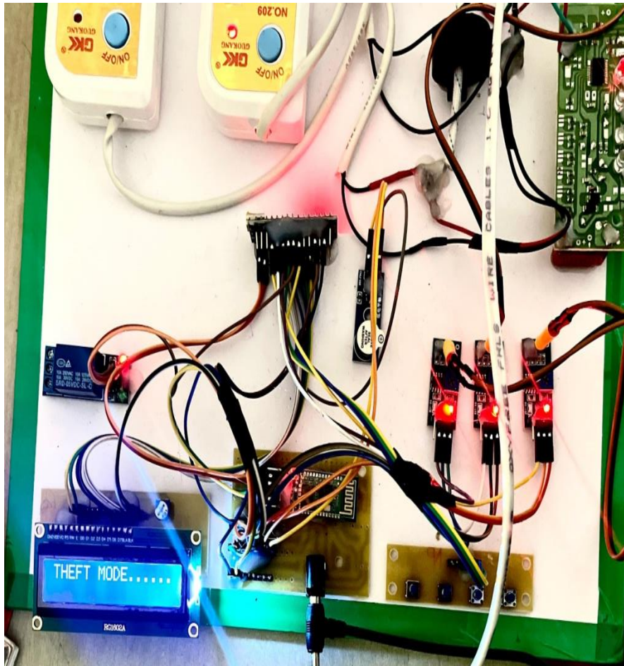
Fig. 4: Real-time monitoring and effective theft detection by comparing consumption at J1 and J2 with the main junction
