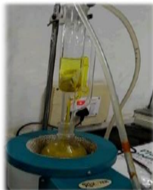
Fig.2: Extraction of Curcumin from rhizomes of turmeric
